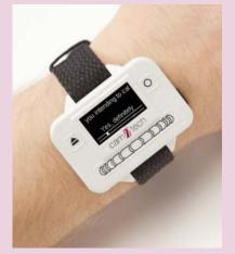
**The PRO-Diary** is a wrist-worn activity monitor with integrated Patient Recorded Outcome Diary. The diary user interface consists of a touch sensitive 'slider' device and two other buttons. It is designed to be easy to operate, and can ask questions of eight different types.
