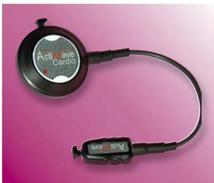
**The Actiwave** family includes ECG/EEG Recorders with 1, 2, or 4 channels and EMG Recorders with 2 channels. The researcher can select the sampling rate from 32 Hz to 1024Hz and the resolution from 8 to 10 bits. Recording times for 128Hz, 8 bit resolution range from 36hrs (1 channel) to 13hrs (4 channels).
