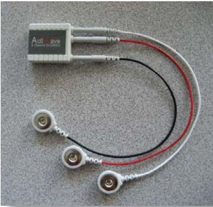
**The Actiwave** monitors have 1mm diameter pins to which slip-on leads are attached. CamNtech supplies two styles of leads. One lead set has touch-proof contacts on one end and 4mm female snap contacts on the other end. The second lead set has custom 1mm female sockets on one end and spring-loaded clip contacts on the other end. Either lead set will attach directly to any ECG, EEG, or EMG electrodes that have 4mm male snap contacts.
