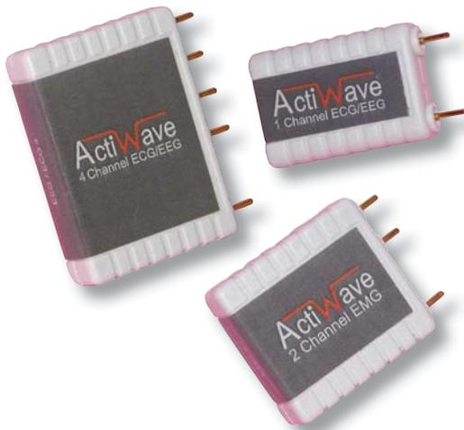
The ultra-miniature size of the **Actiwave** family of wave recorders makes them a practical, unobtrusive alternative for monitoring sleep. Weighing 10g or less, the Actiwave can be adhered to the skin with little risk of detaching. With a thickness of 8mm, they can be placed in a convenient location on the body without creating discomfort.
