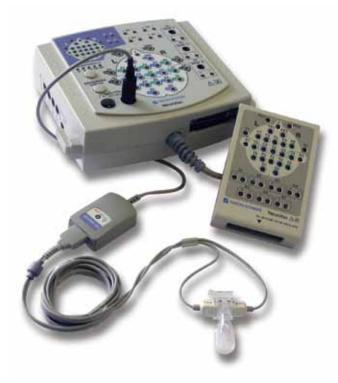
20 uni-polar and 14 bipolar inputs. With built in SpO<sub>2</sub> this amplifier combines economic sense with flexibility.
