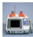
ECG waveform and annotated data from 8 seconds before to 12 seconds after defibrillation is saved automatically.
